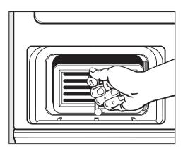
Pull the condenser unit out of its housing by the handle.
